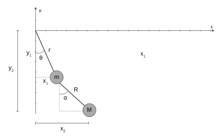
It is again useful to describe the positions of both of the pendulum bobs by the angles as shown in the picture. For the first bob, the x and y -coordinates, expressed in terms of the angle  $\theta$ , are as follows:
